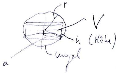
$$V = \text{Vol}_{\text{zyl.}}(h, r) \left( = h \cdot \underbrace{\sqrt{r^2 - \left(\frac{h}{2}\right)^2}}_{a^2} \pi \right)$$
