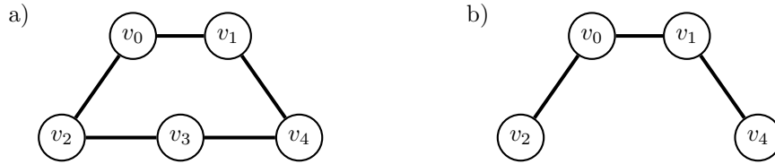
Figure 4: In graph a), the vertices v_2 and v_4 are compatible, because their distance is two. In the graph shown in b), vertex v_3 is removed. The removal of v_3 destroys the shortest path between v_2 and v_4 with a distance of three. The vertices v_2 and v_4 have become incompatible through the removal of v_3 .
